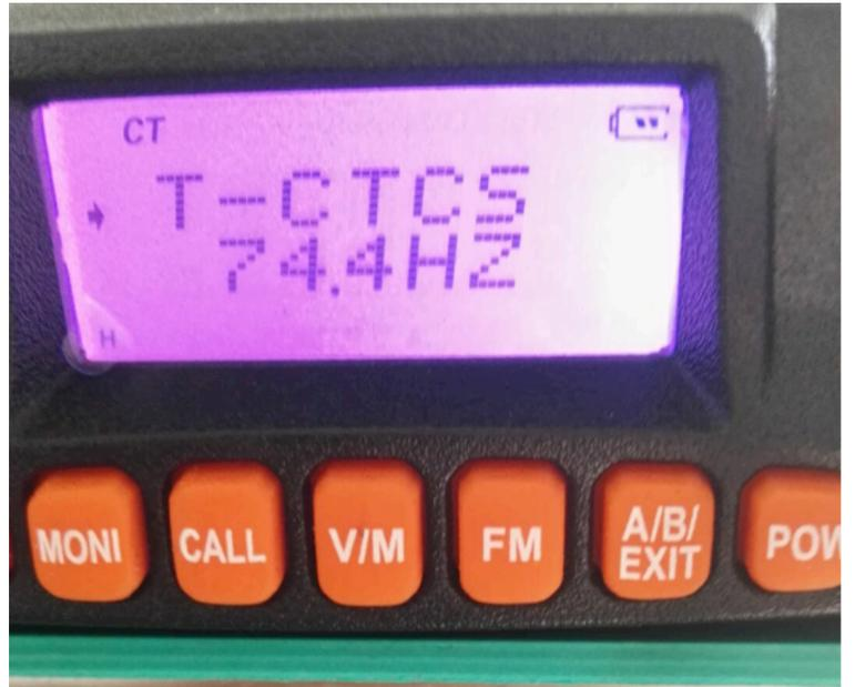
3: Enter MENU 43 REP-M and select CTDCS for two mobiles – this will require the repeater forwarding (X-Band Repeat) to activate once the confirmed PL signal (CTCSS or DCS) is received will transmit it on.
