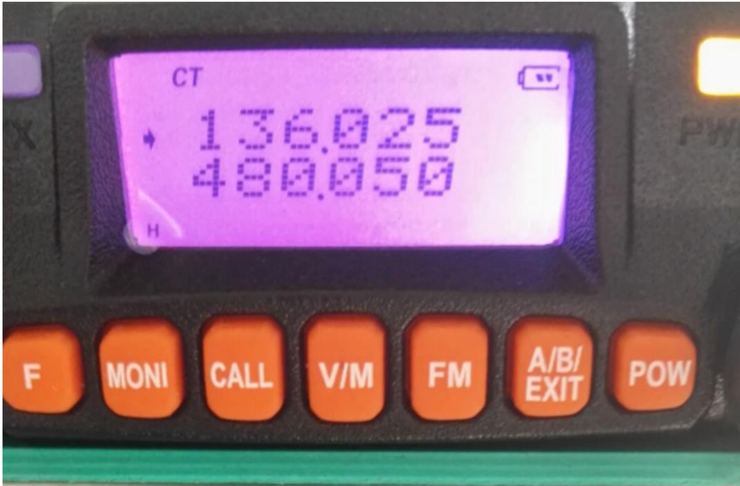
2: On **both** BTECH mobile radios set the PL Tones with MENUS 11 and 13. In this example set R-CTCS (Menu 11) to 74.4Hz and T-CTCS (Menu 13) to 74.4Hz
